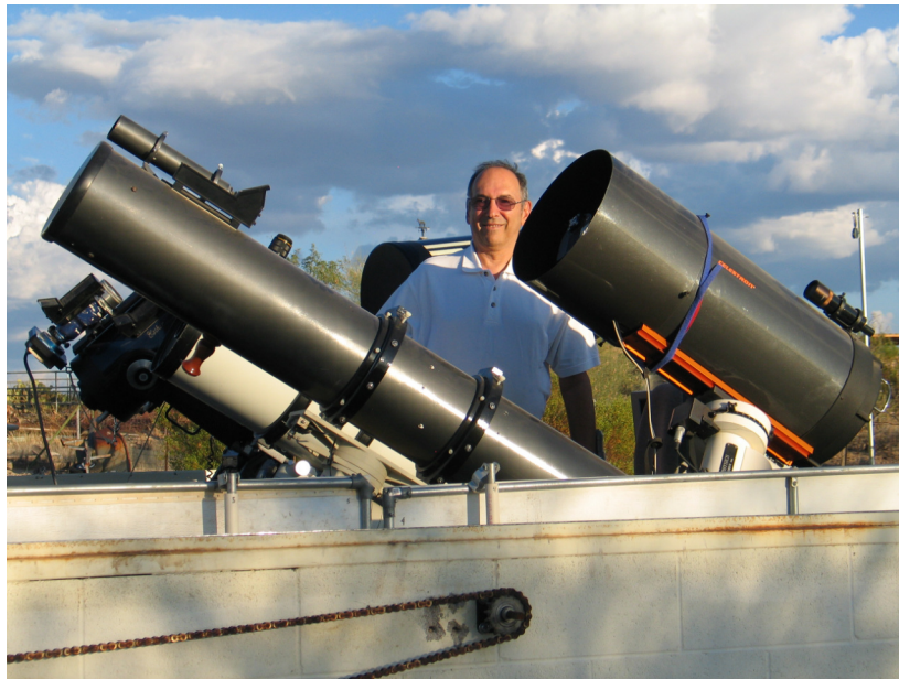
Two of the telescopes Dave uses in the observing at Jarnac Observatory. The telescope on the right is used for astrophotography (he doesn't do much of anymore) and the telescope on the left is Pegasus. It is used for visual observation. It is the highest quality telescope he has. The mirror was made by Aleka Herring, one of the most prominent telescope makers in the last century. Picture taken by Wendee Levy.
