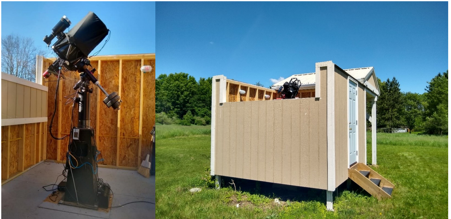
All images were taken with the 10" f/8 Riche-Cretien telescope. The camera is a ZWO asi071mc PRO and the mount is a Losmandy G11.
