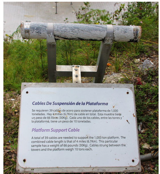
Figure 3: Platform support Cable
