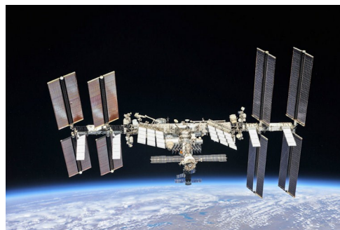
A complete view of the ISS as of October 4, 2018, taken from the Soyuz capsule of the departing crew of Expedition 56 from their Soyuz capsule. This structure was built by materials launched into orbit by 37 United States Space Shuttle missions and 5 Russian Proton and Soyuz rockets, and assembled and maintained by 230 spacewalks, with more to come! Credit: NASA/Roscosmos More info: bit.ly/issbasics
